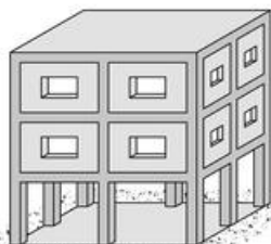
(a) Stiff and strong upper floors due to masonry infills
